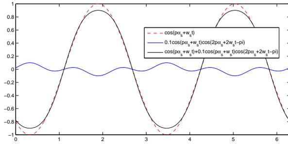
Fig. 1. Illustration of the air-gap radial flux density flattening due to even order saturation permeance waves.
