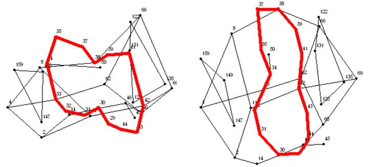
Fig. 2. Deflection shape of tested motor at  $f_s(38/2 + 4) = 23f_s$ , with  $f_s = 30$  Hz (no load case), captured at two successive moments.
