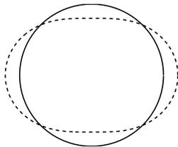
Fig. 2. Example of a 2-order ( $m = 2$ ) rotating force wave coming from the Fourier series development of radial air-gap Maxwell forces distribution. The fundamental difference with the deflection shape of the stator elliptical mode in Fig. 1 is the fact that the exciting force nodes are rotating, whereas the mode deflection nodes are steady, fixed according to the maximal stiffness points of the structure.
