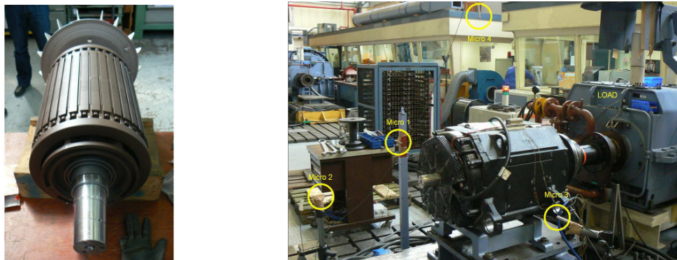
Figure 6: (Left) Rotor prototype with Z_r=36 slots. (Right) Experimental set-up.
